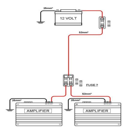
Factory dual battery systems may not have any fuse (or protection) between the batteries. It is up to the competitor to prove the original installation of his vehicle.
