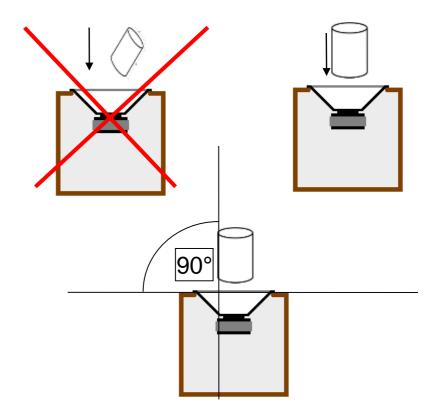
The protection of speakers will be judge with a cylinder and with an angel from 90° between cylinder and the speaker mounting panel at the center position The cylinder should not be able to touch the **MEMBRAN**, but NO deduction when touching the **SURROUND**!
